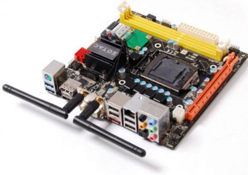
Assemble the perfect small form factor system for all your computing demands with the flexible ZOTAC® H61-ITX WiFi mini-ITX platform. The ZOTAC® H61-ITX WiFi supports socket LGA1155 2nd generation Intel® Core™ family processors with turbocharged Intel® HD Graphics to let users select the perfect amount of processing power for their needs – whether it is dual or quad-core, with or without Intel® HyperThreading™ technology.
